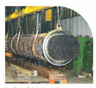
In refineries, Re-boilers are used as a type of shell and tube heat exchangers to reheat the condensate products at the bottom of distillation columns and return them vaporized to the distillation columns. Re-boilers are also designed and manufactured by MAPNA Boiler.
