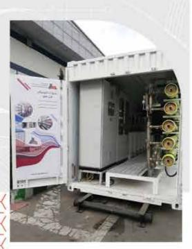
Various pretreatment units are available designed earlier which consists of pressurized sand filter, Ultrafilters (UFs), self-cleaning screen filters, disk filters. In all the water package products, Reverse Osmosis (RO) plays the part of water desalting and the process of demineralized water production is on Electro Deionization system (EDI). All systems are supported by electric and control panels and there is the possibility of remote monitoring using GPRS technology if requested by a client.
