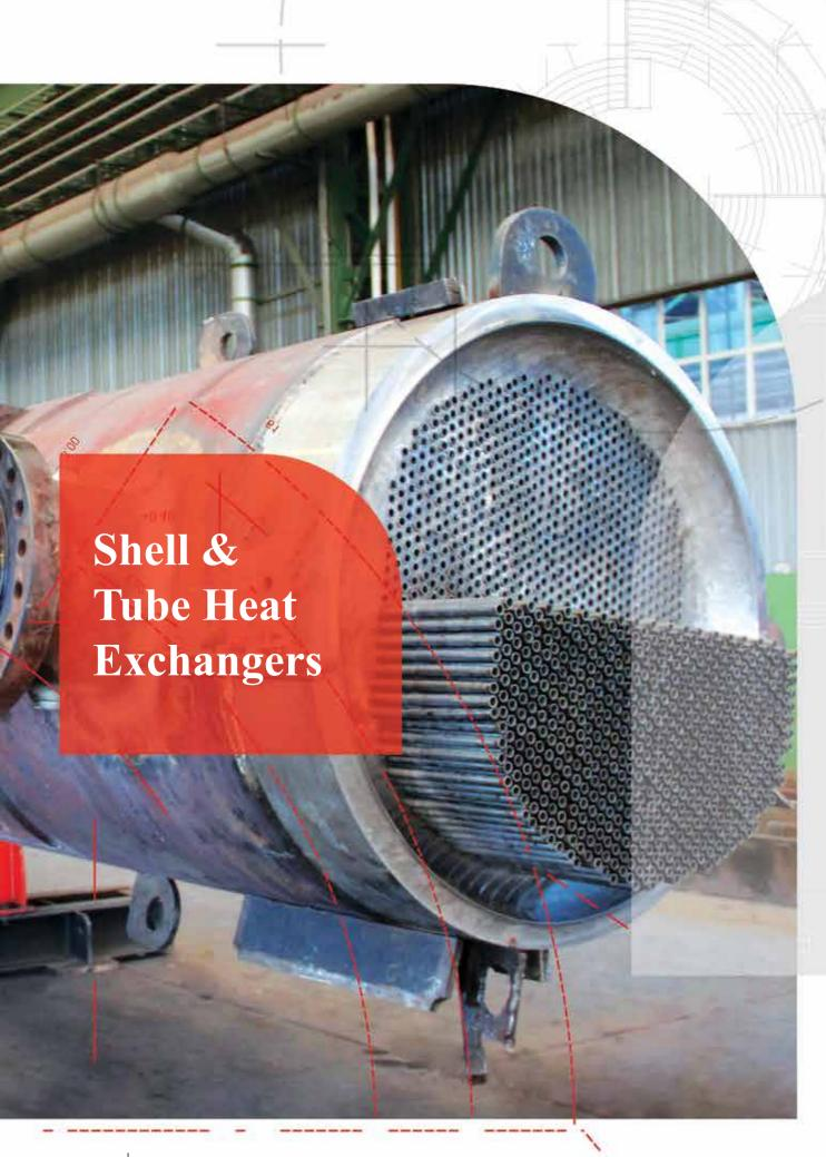
Shell and tube heat exchangers span a vast range of applications in the downstream and upstream industries of oil, gas, petrochemical and power plants and food industries. Resting on experts' knowledge as well as modern manufacturing tools and machines, MAPNA Boiler Company is ready to present services in the field of design, construction and maintenance (re-tubing) of such heat exchangers.
